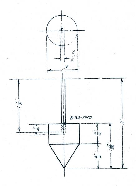
PLUNGER FOR PENETROMETER Material-Red Brass
