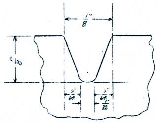
Enlarged Four Times DETAIL OF GROOVES
